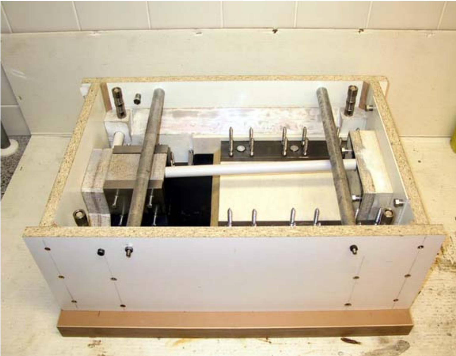
Mold for the base. This base will be case upside down. Note the screws sticking up from the metal parts--that's how they're anchored into the epoxy matrix...
