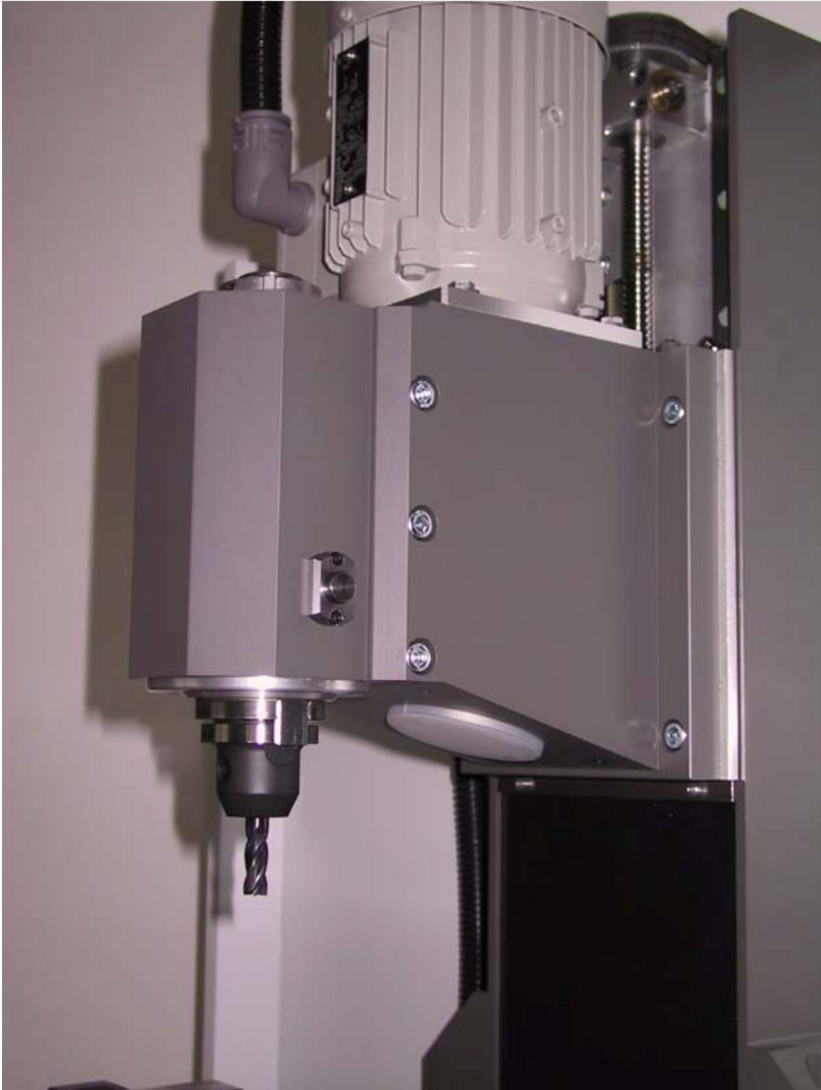
Not sure of the taper. The text mentions SK30. That's a release button on the side, so there must be a compressed air drawbar with bellville's or some such...
