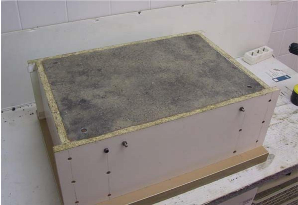
The Epoxy Granite Has Been Poured Into the Mold...
