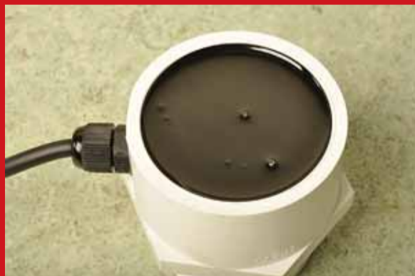
Photo 15: when cured and removed from the jig, this is what it will look like (hopefully without the air bubbles, although these won't affect operation). The top of the potting compound is just below the top of the fitting.
