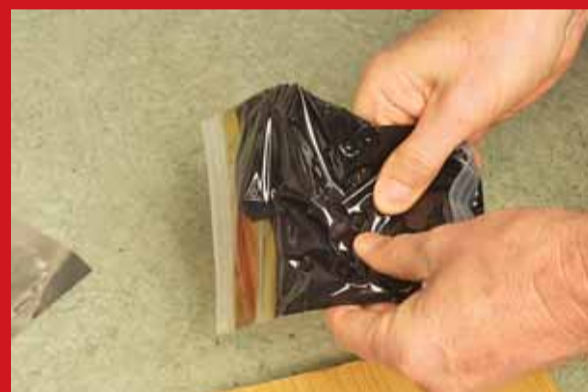
Photo 11: the potting mix comes in a two-part pack which must first be combined and then thoroughly mixed before use. You need to knead it! On a cool day, this can take quite a few minutes to do, but if you don't mix completely, the compound may not cure properly.
