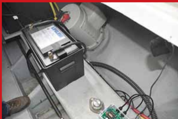
Photo 24: the location for the driver unit is just as important as the transducer. It must be one which can NEVER interfere with any boat operation and one which won't be stepped on if you need to get into the area. Just as important, it must be one which won't be swamped by bilge water, despite the IP65 case.
