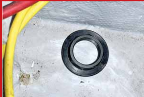
Photo 19: move the empty flange around the hull to determine the best transducer mounting position. When you're happy with your choice (see the text), roughen the fibreglass as you did the black flange – for the same reason. Here the flange is sitting in place but not yet glued.
