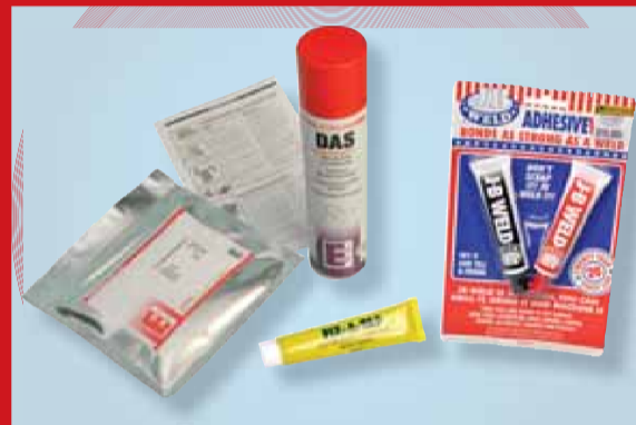
Photo 1: before we get under way, here are the chemical products we're recommending. On the left is the Electrolube polyurethane potting compound, with instructions and the Electrolube silicone mould release. Centre is the Fix-A-Tap waterproof lubricant (available from hardware stores and pool shops) while on the right is the J-B Weld 2-part epoxy glue. It's not easy to get – but it works!
