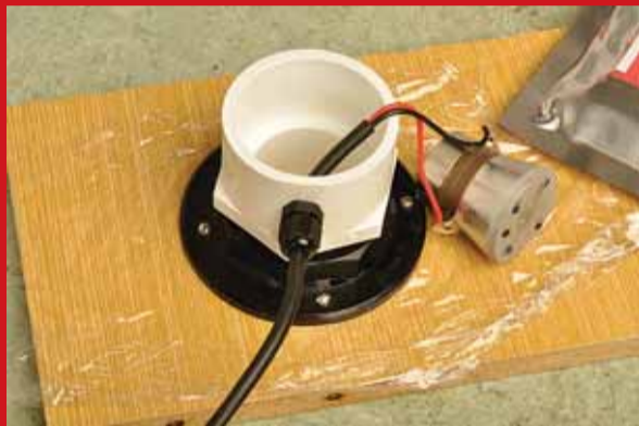
Photo 10: remove the transducer and screw the empty pipework into the nut. Make it firm, but not so tight that it bites into the cling wrap. You're now just about ready to pot the transducer so make one last check that your solder joints are perfect – once potted, it's very hard to remove !
