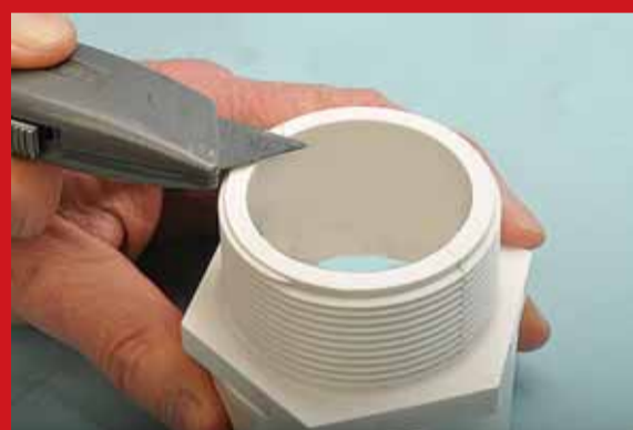
Photo 3: Unfortunately, on the threaded end there were some moulding dags – we need the base perfectly flat, so we trimmed these off with a sharp knife and then smoothed it off with some sandpaper.
