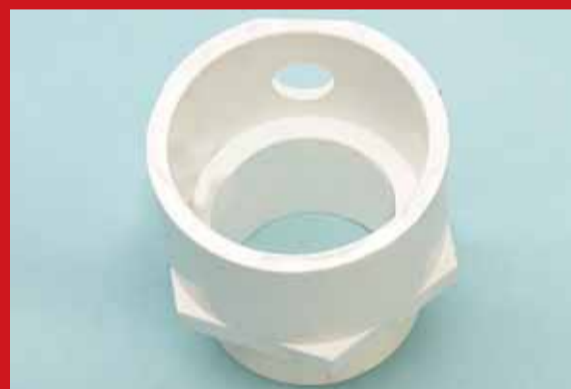
Photo 2: here we've filed a flat on one side of the 50mm BSP male valve socket and drilled a 12mm hole, both of which are needed to accommodate the 6.5mm cable gland through which the wires pass from the driver to the transducer.
