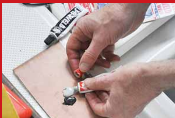
Photo 20: did someone mention glue? We're recommending J-B Weld to secure the flange to the hull. It's not that easy to buy (try your local hardware store as distinct from the big chains) and it's not cheap – but it sticks like the proverbial.
