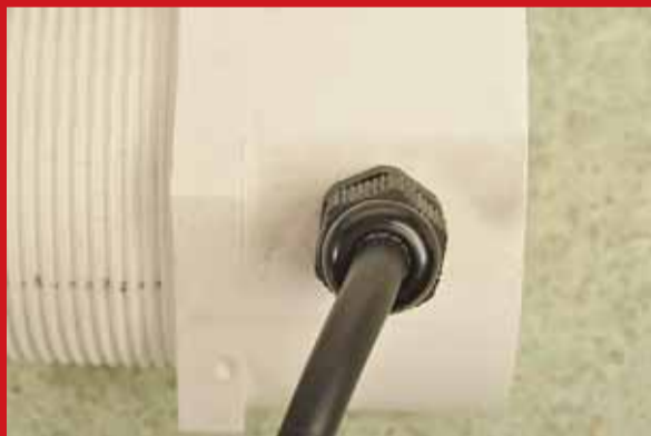
Photo 5: the 6.5mm cable gland, when tightened up later, makes a completely waterproof entry point for the flexible cable from the driver unit. The recommended cable is double-insulated but still highly flexible.
