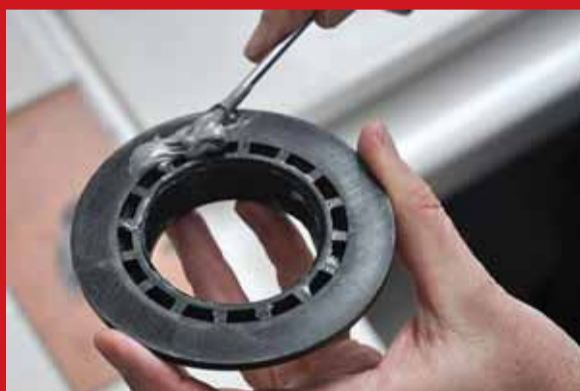
Photo 21: apply a good layer of mixed glue all over the roughened base of the flange, again making sure you don't get any on the thread. You have quite a while before it starts to cure, so take your time!
