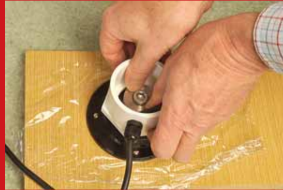
Photo 13: now push the transducer hard down, into the potting mix, face down. About now you might find out that overfilling with potting mix makes a nice mess of your thumbs . . . try to get the transducer as centrally located in the tube as possible, although it's not vital. Pull the cable back through the grommet until about 10mm of outer insulation is showing inside, then tighten the nuts.
