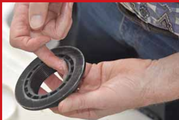
Photo 18: it's important that glue doesn't get into the thread, where it would clog it up. We smeared a good coating of Vaseline right around the threads – make sure it doesn't get on the bottom of the flange where you want the glue to take!
