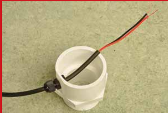
Photo 4: next, we passed the end of the flexible 2-wire cable through this cable gland, leaving plenty of free wire on the inside. Leave the cable gland nuts loose at this stage to allow the cable to slip in and out.
