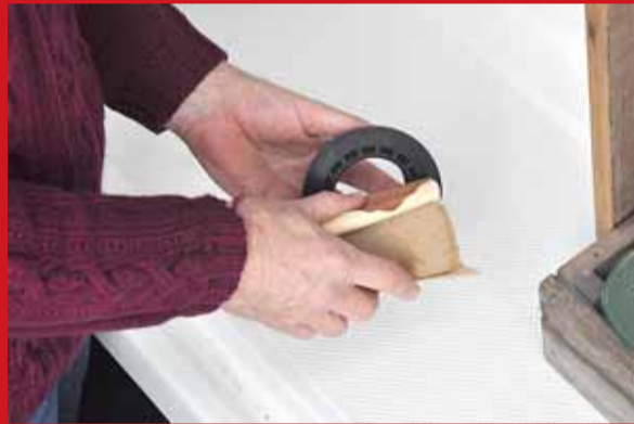
Photo 17: now we're moving onto the installation in the boat. After you remove the black plastic flange from your temporary jig, roughen the bottom with some coarse sandpaper. This is to give a good 'key' for the adhesive to ensure it won't vibrate loose when fixed to the boat hull.
