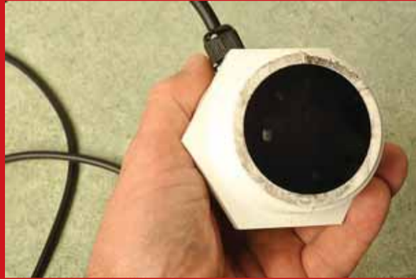
Photo 16: and here's what it looks like from the underside (the bit that contacts with the boat hull). The 'rough' edge on the socket is actually a smooth edge – we removed some thread ends with sandpaper.
