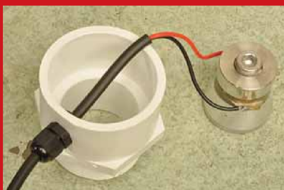
Photo 6: next, we soldered the two bared ends of the cable to the lugs on the side of the transducer (disconnect from the driver unit first!). Make sure these solder joints are good 'uns, because once potted, you won't be able to get at them!
