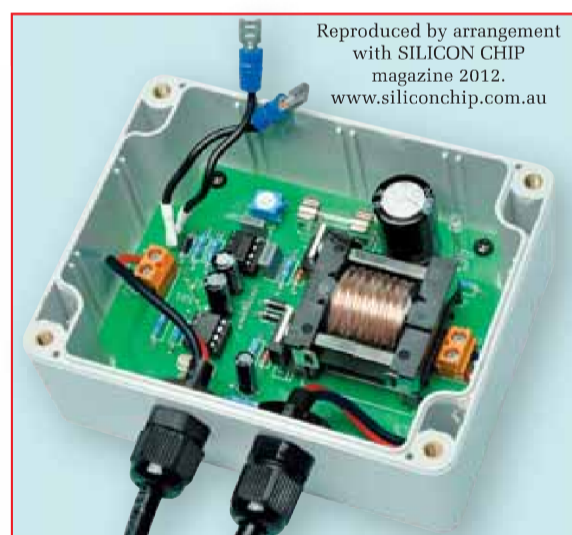
Driver board mounted inside the case. Do not apply power to the completed unit unless the transducer (which must be fully encapsulated) is connected – see text.
